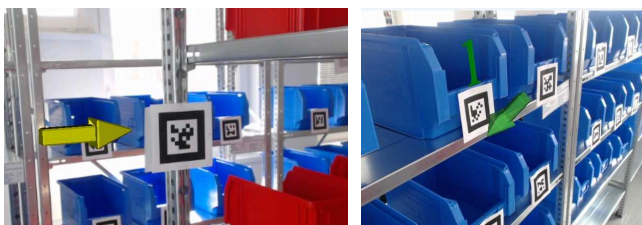
Fig.1. Navigation by augmented reality using markers
