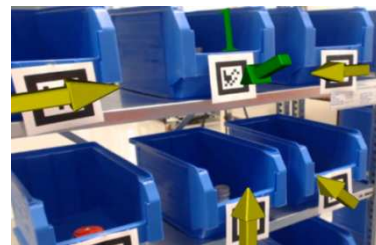
Fig. 3 Directional and order picking information displayed via augmented reality
