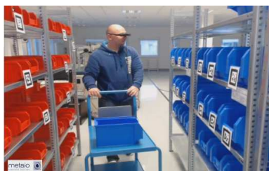
Fig. 5 Picking items with augmented reality
