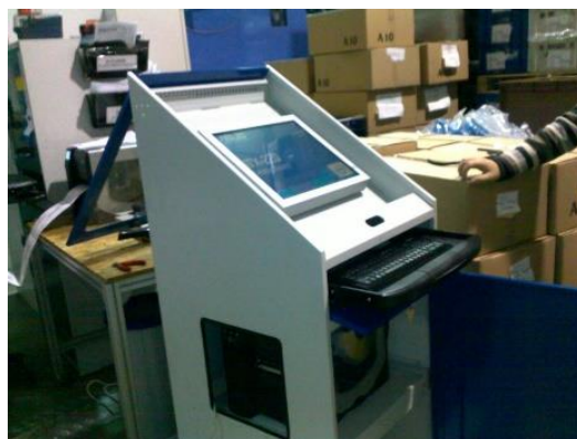
Fig. 9. Workplace with computer station for registration of manufacturing processes' progress
