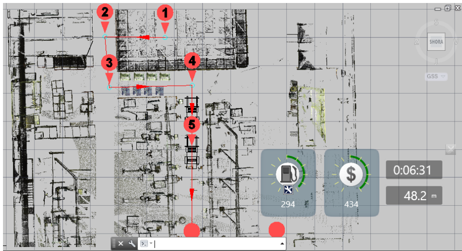
Fig 5. Material flow analysis in AutoCAD with Factory Design Utilities. Point cloud is used as an underlay
