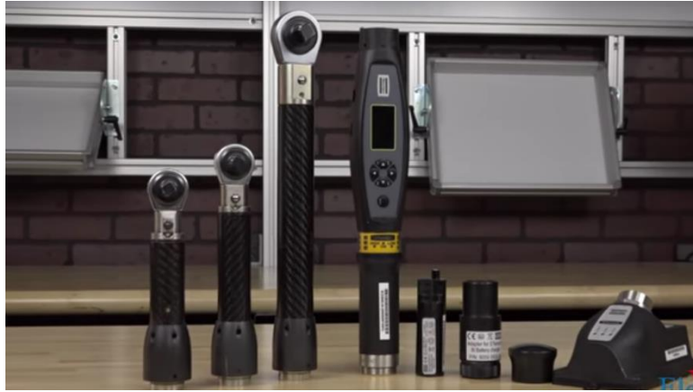
Fig 2. The example of transducerized hand-held torque wrench [7]
