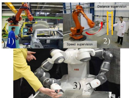
Fig.1. Examples of the cooperation modes: 1) Hand guided, 2) Speed and separation monitoring, 3) Power and force limiting
