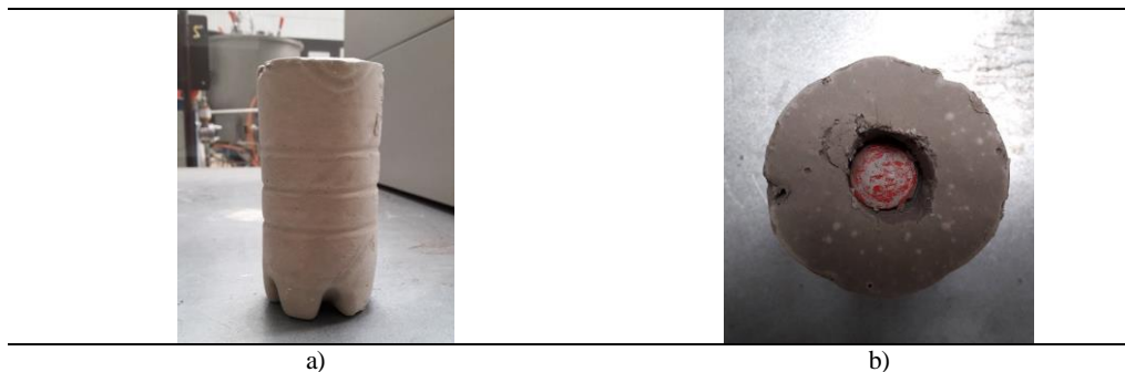
Fig. 2. a) Gypsum mold; b) Gypsum mold with the physical model of the cylinder
