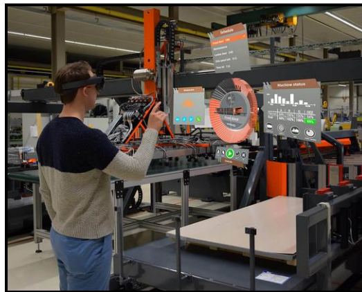
Fig. 1. The worker sets up a production line with augmented reality
