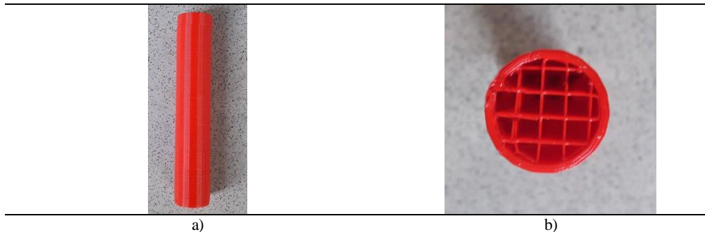
Fig. 1. a) Physical model of cylinder; b) Infill ratio of printed cylinder
