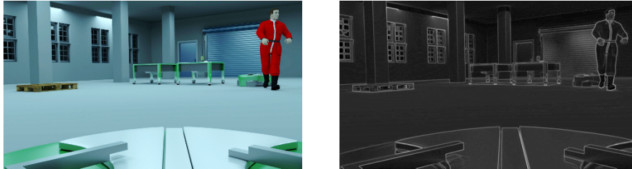
Fig. 5: Image processing from RGB picture to grayscale picture with detected sharp edges
