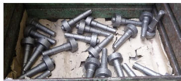
Fig.3. Typically rotational part for using mechanical gripper
