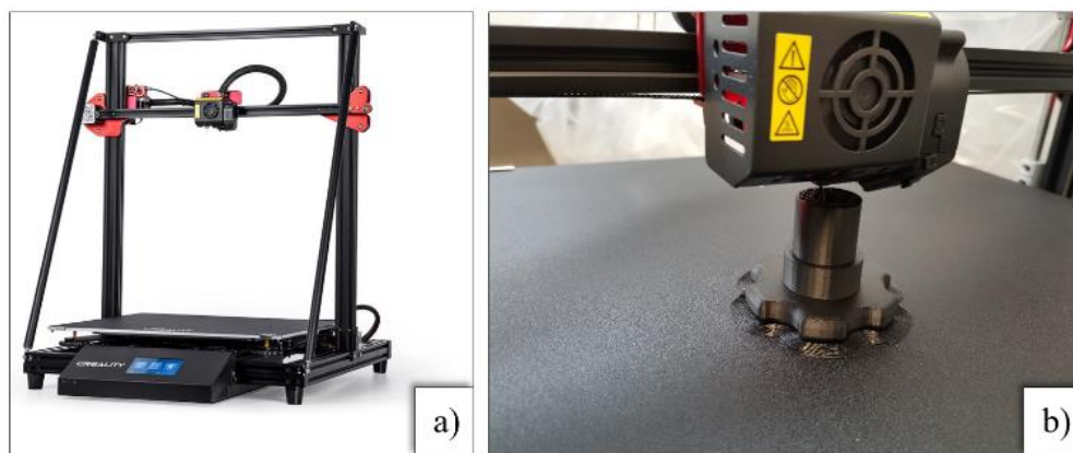
Fig.1. Creality CR-10 Max the 3D printer (a) [7], Process of 3D printing (b) (main author)
