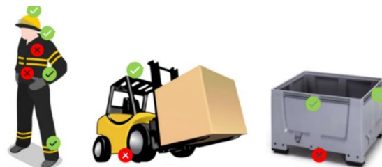
Fig. 3 Appropriate / inappropriate placement of tags on objects
