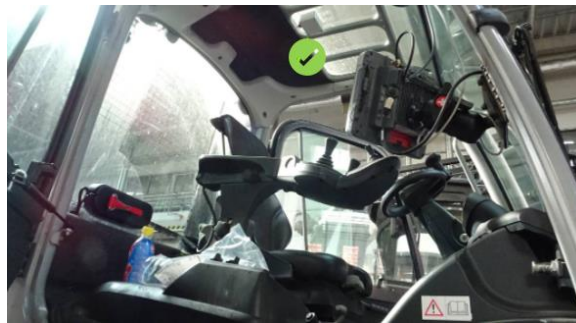
Fig. 2 Example of placing a tag on a forklift roof
