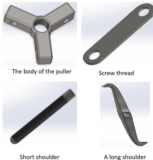
Fig. 2 Puller body parts
