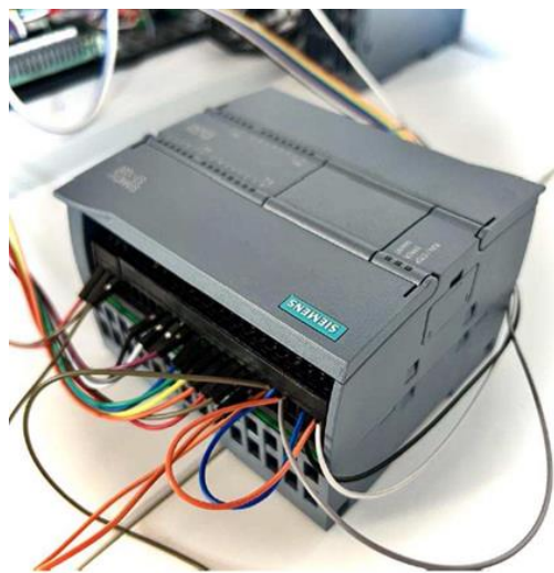
Fig. 2 PLC Simatic S7-1200
