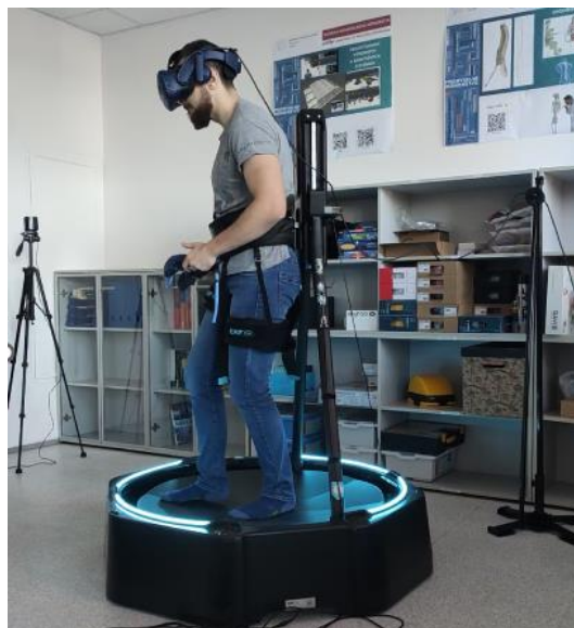
Fig. 2 Omni-directional VR treadmill (authors).
