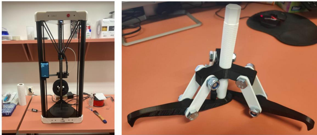
Fig. 7 3D printing of a bearing puller
