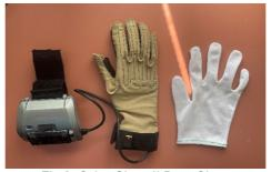
Fig.2. CyberGlove II Data Glove
