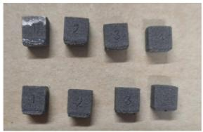
Fig. 2. 3D printed cubes using the SLM method
