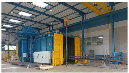
Fig. 5. Automatic blasting machine
