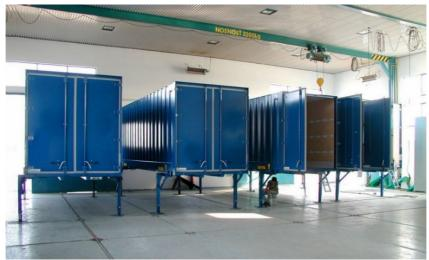
Fig. 1. Exchangeable superstructure
